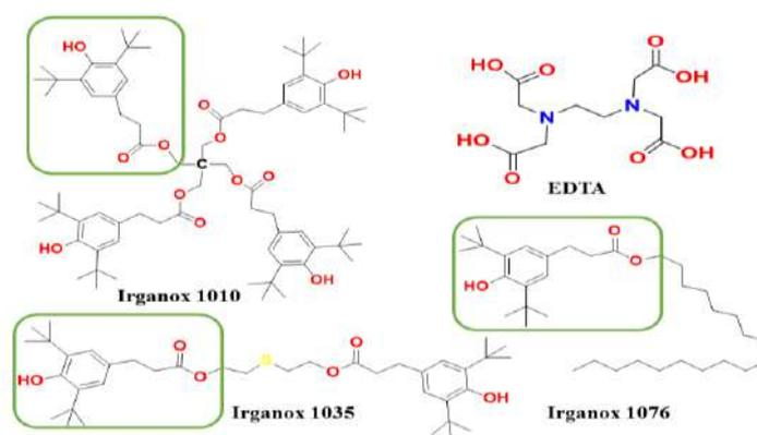
**Fig.1** (2D chemical structure of EDTA and various Irganox types which have the same base unit)
